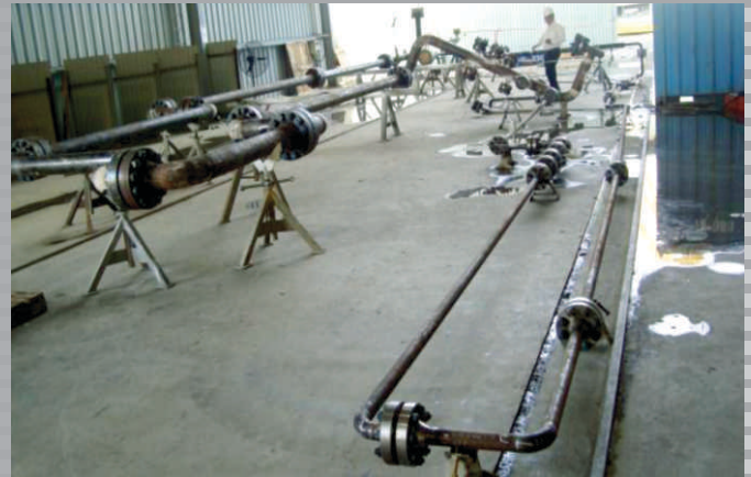
Hydrostatic test for Flowline at 5560 psig
