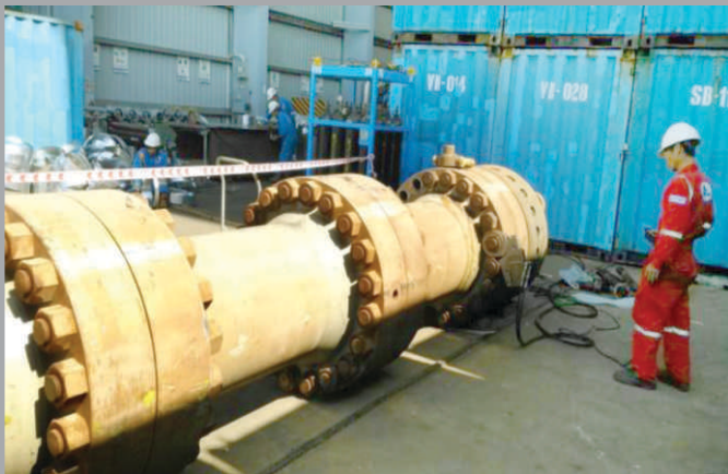
Hydrostatic test for HP Riser at 22500 psig
